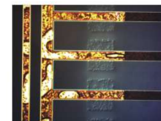
Conducting particles 20X DIC
